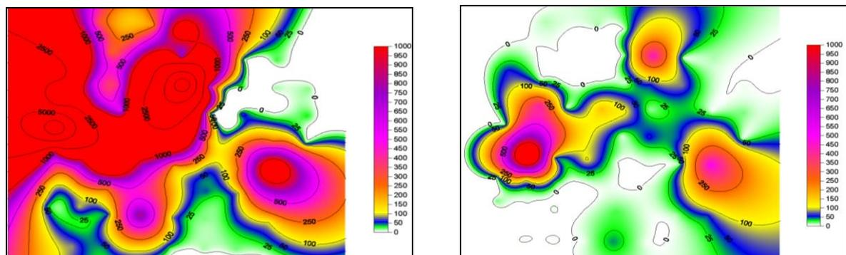
Figure 2: PID monitoring pattern at the start and end of the SVE works.
