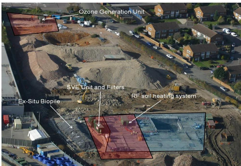
**Figure 1. Aerial photo of the remediation layout during the remediation project – Areas in red underwent ozone sparging; the area in blue underwent soil vapour extraction.**
