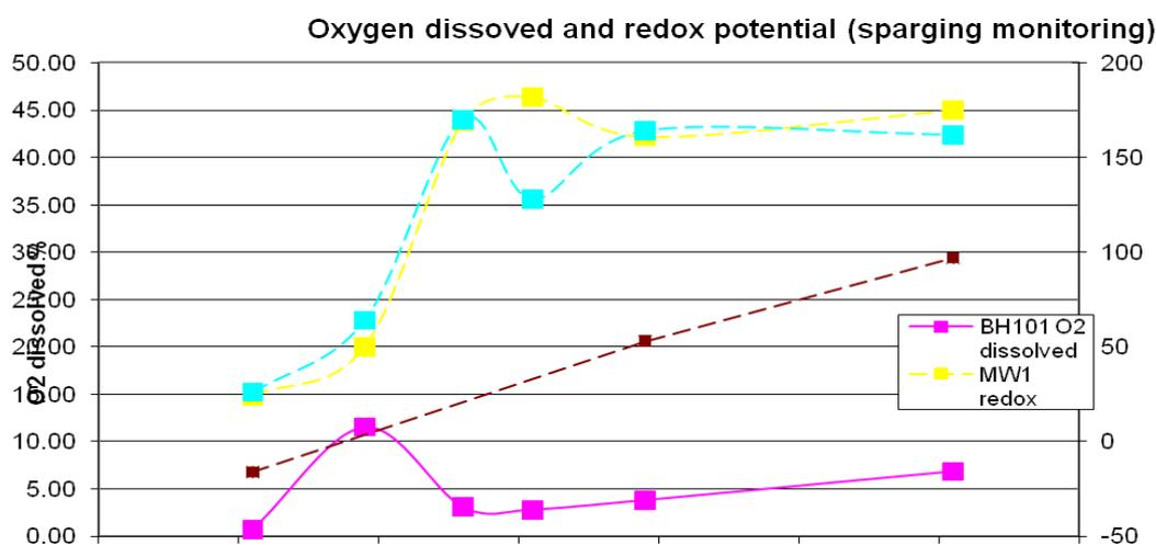
**Figure 3 Increase in dissolved oxygen and redox potential during ozone sparging of the central area.**
