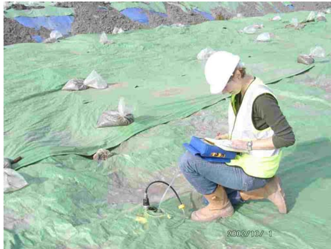
Plate 8.1: Measuring gas concentrations
